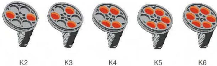
The qty of spring return pneumatic actuator can choose economic qty according to the valve torque, the assembly position of different springs' qty according to the above table (red part is position for putting springs' )
